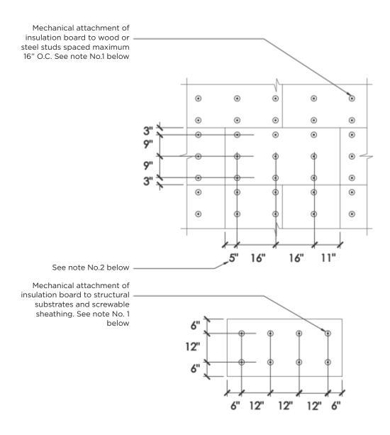
NOTE 1: The above fastener spacing pattern shall be provided as a minimum, faster type. Spacing and depth of the penetration shall be determined by the design professional to meet specific job requirements.
